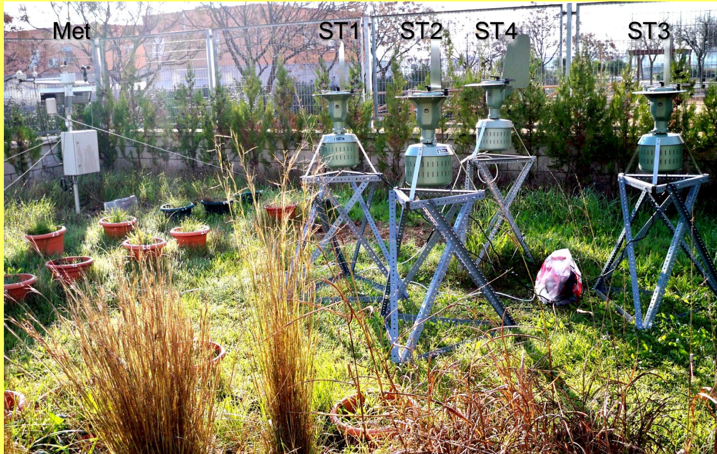
Meteorological station on the left and the four spore traps at the experimental garden on the right
