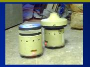
Both samplers suck air at 10 l/min. Sampling was done during 10 min.,
